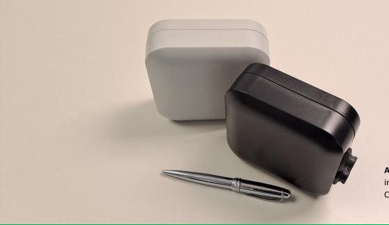
**ARC–Landing** includes one Primary for installation onto the UAS and four Cooperating radar for the landing area.
